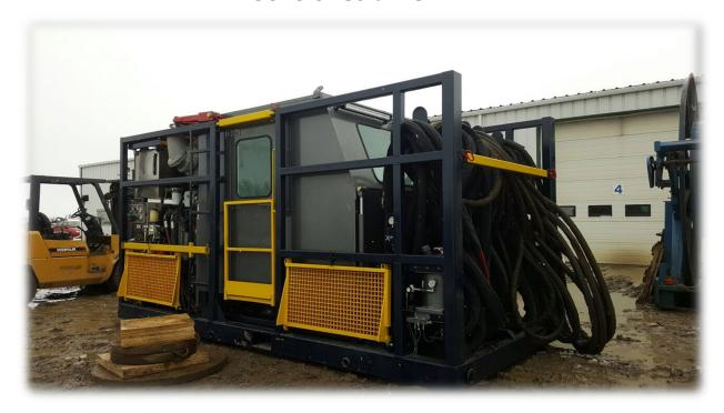
Mounted on the deck is an automated Strap lift operator's station. It extends several feet above the tubing reel to give the operator a clear view of the wellhead and the activity around it. It is temperature controlled so the unit can be operated comfortably in temperatures from -40C to +50C.
