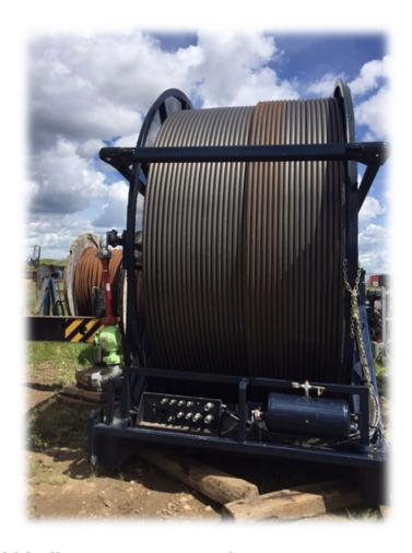
The reel uses an S&S offset open spoke type of construction with square and rectangular steel tubing. The 80" core consists of a rolled steel tube and lateral cross support beams. The tubing reel is mounted on heavy duty roller bearings in a steel frame that is complete with level line to spool the tubing evenly. The reel has a dual ported drum with 10K Rotating Joint and 1502 Treatment Iron and 3" 15K valves.
