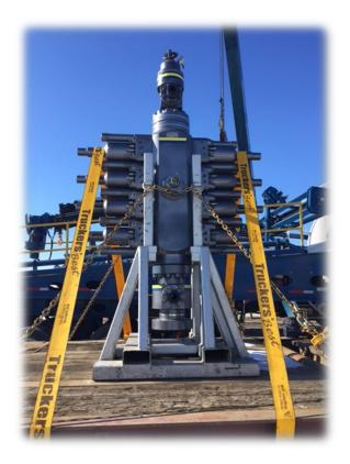
This unit uses a Nexus 5" 10k Quad Hydraulic BOP system, which has Quick Lock Hydraulic Actuators, complete with fire retardant hose package.
