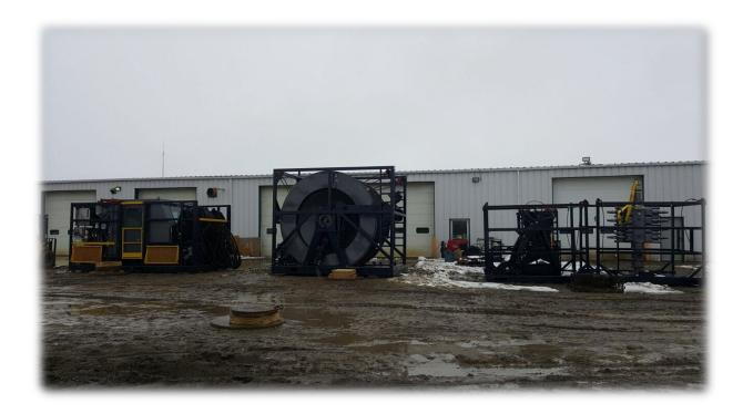
Titanium's' Off Shore Skid mounted Coil Tubing Unit consists of four skids which can be used for land or sea well intervention. This Unit has applications for deep Vertical or horizontal completions and workovers.
