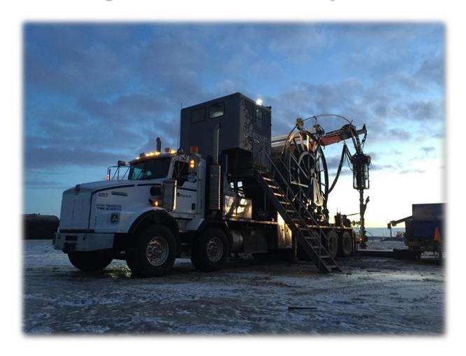
Titanium's Intermediate Body Job Coil Tubing Unit mounted on a Kenworth twin steer, tridrive chassis. This Unit has applications for horizontal completions and workovers up to 4500 meters, and can carry tubulars up to 2.38" O.D. Our injector heads have 150 feet of umbilical for long reach to minimize moving around on pad sites.
