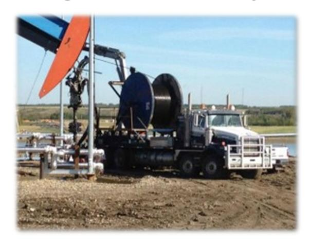
Titanium's Instrumentation Body Job Coil Tubing Unit is mounted on a Western Star twin steer, tri- drive chassis. This Unit has applications for SAG-D horizontal completions and workovers up to 4500 meters, and can carry tubulars up to 2 3/8" O.D. Our injector heads have 150 feet of umbilical for long reach to minimize moving around on pad sites.
