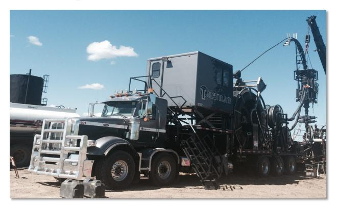
Titanium's' E-Coil Tubing Units are fully integrated units that are mounted on Peterbilt twin steer, tri-axle drive chassis. These Units have applications for deep horizontal completions and workovers, and have the advantage of carrying large diameter tubulars, while keeping the overall footprint small for congested well pads.
