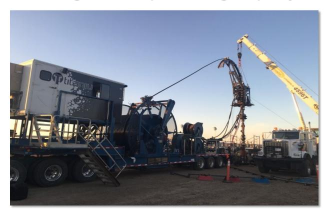
Titanium's' deep Trailer Coil Tubing Unit is a pulled by a Peterbilt single steer, tri- drive chassis with a full wet kit. The Coil Unit is on an Atoka Tri-Axle Trailer and has Available Jeep and Booster package to make legal weights. This Unit has applications for deep horizontal completions and workovers, and have the advantage of carrying large diameter tubulars, and 150 feet of umbilical for long reach to minimize moving around on pad sites.
