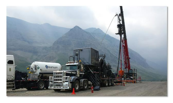
Titanium's deep body Job Coil Tubing Unit is a fully integrated coil tubing units are mounted on Peterbilt twin steer, tri-axle drive chassis. These Units have applications for deep horizontal completions and workovers, and have the advantage of carrying large diameter tubulars, while keeping the overall footprint small for congested well pads.
